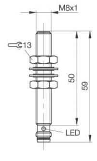
**Inductive Sensors** BES M08MI-PSC40B-S49G M 8x1 x 59 normally-open Sn=4mm quasi shielded
